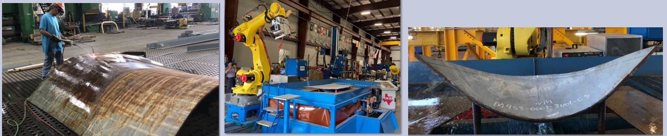
(l) Ingalls' current forming process using line heating; (c) Automated plate-shaping system developed by Navy ManTech; (r) Plate formed by Navy ManTech system in approximately 4 hours; the manual process to form the same plate takes nearly 54 hours
