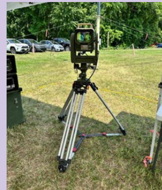
(r) The TALON Transceiver is a crucial component of the TALON system, enabling high-speed data transmission over FSO links. With a data transfer rate of up to 800 mbps, it ensures efficient connectivity for mission-critical operations
