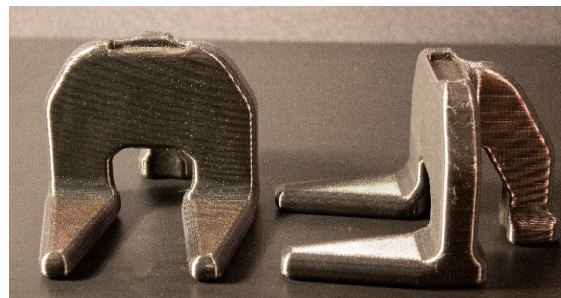
Figure 2. Shadow Jackstand holds the Army aircraft up and allows a single person to change the tire significantly reducing time required to perform the maintenance task. Read more on p. 4.
